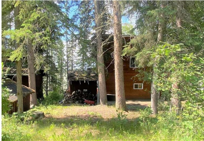
Figure 3: Firewood stored too close to structures provide ignition points and fuel for wildfires.
